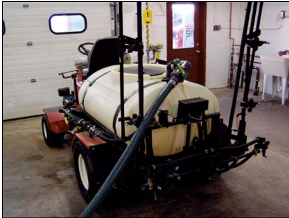
2 inch transfer line connection allows fast, spill free fill rates of 100 GPM or better
